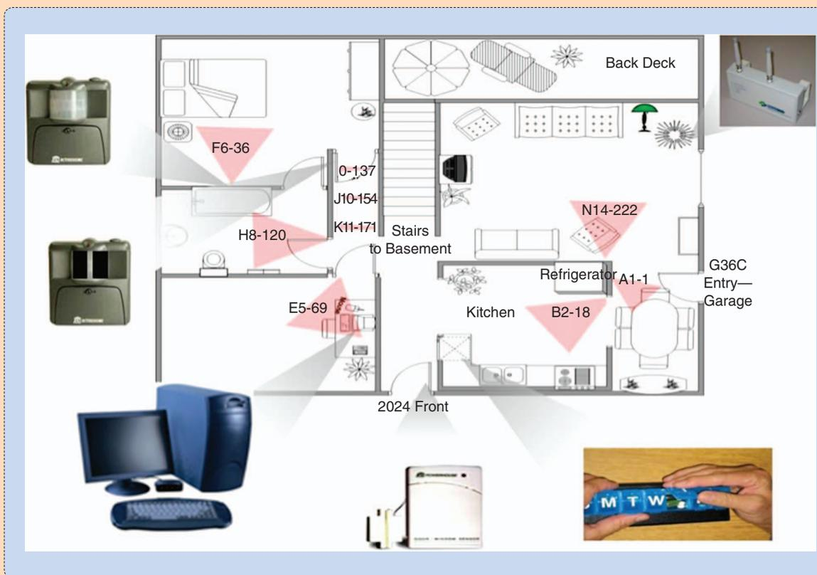
**FIGURE S1** A variety of sensors used in the ORCATECH participants' homes. These include passive IR motion sensors for activity monitoring, reduced field-of-view motion sensors for measuring walking speed, computers with software for measuring cognitive function and motor speed, door switches, phone sensors, and Bluetooth-enabled medication monitoring [S2].
